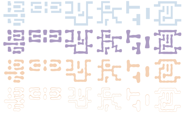
Figure 5: Visualizations of results. Rows from top to bottom are: target layouts, optimized masks, printed wafer images, and PV bands.
